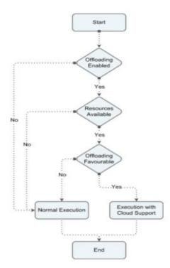
Fig. 2: Process of computation offloading
